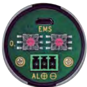
Thermalert 4.0 supports 2-wire loop
