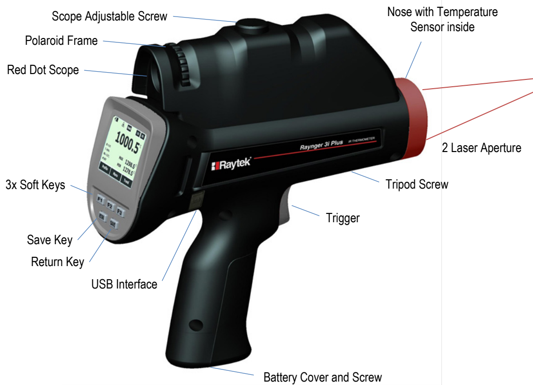
Figure 3: Portable Thermometer with Scope
